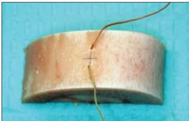
**Fig 3** Microthermocouples in bone segment.
