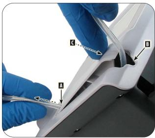
14. Attach the small end of the irrigation tube A to the handpiece irrigation fitting, following the instructions that came with your handpiece. Attach the irrigation tube to the motor cable at evenly spaced intervals using the AHP-03 clips provided in the AE-24 tubing set bag.
