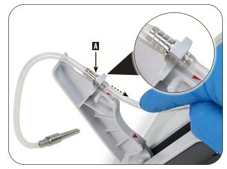
**12.** Following the next red arrow on the pump door, thread the peristaltic tube segment through the bottom slot **A** on the pump door.
