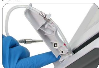
13. With one hand, pull the irrigation tube firmly from the bottom of the pump door ⚠. Use the other hand to guide the irrigation tube into the notch ☒ on the console while closing the pump door ☒.
