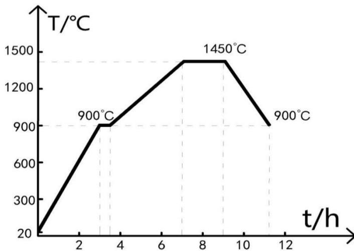
**Stain & glaze sintering process** ( To avoid subfissure happening on bridge, the heating rate for bridge stain & glaze sintering must go down to 30°C/min)
