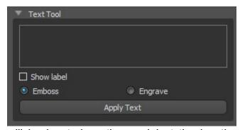
It is first necessary to check whether the correct model is selected. If the model is set as invisible at this point in time, the user is notified of this when he or she tries to insert a label on it. The text is inserted into the editing field. At this point, an auxiliary display of the text entered is also shown in the 3D display window. The text
