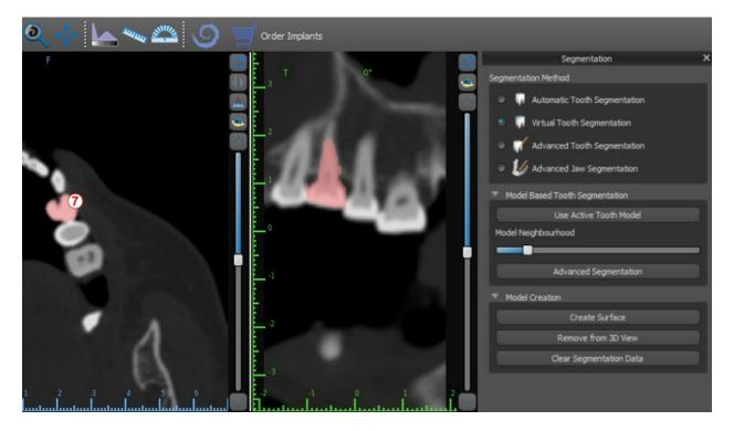
If automatic delimitation of the tooth fails, it can be selected in the data using the virtual tooth manually positioned in the data via the "Virtual Teeth > Add Tooth" option from the main menu. After positioning the model, perform the "Use Active Tooth Model" action for the designated data on the basis of the tooth model entered. Using the "Model Neighbourhood Parameter" you can perform a slight correction of the area around the positioned model which is selected.
