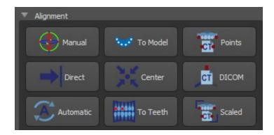
If the model is already aligned with respect to the data, the "Direct" should correspond to the correct position of the model. For STL models created with different software than Blue Sky Plan®, use the "DICOM" alignment. "Center" places model into middle of the scene without performing any rotation.
