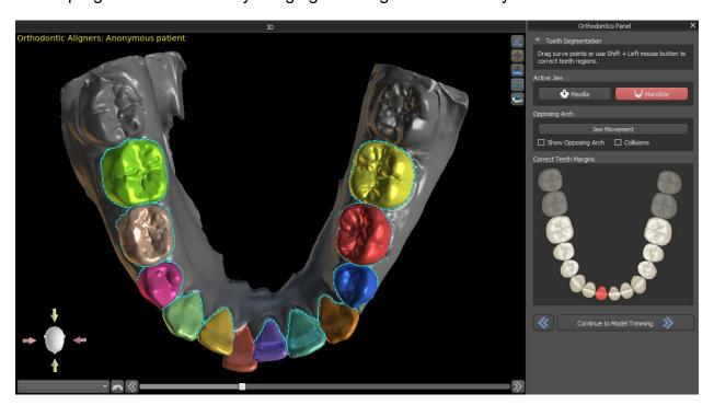
After the automatic segmentation, you can adjust the detected gingival margin of the active/selected tooth by dragging the control points of the curve, or by manually drawing a part of the curve on the model while holding down the "Shift" key and left mouse button simultaneously.
