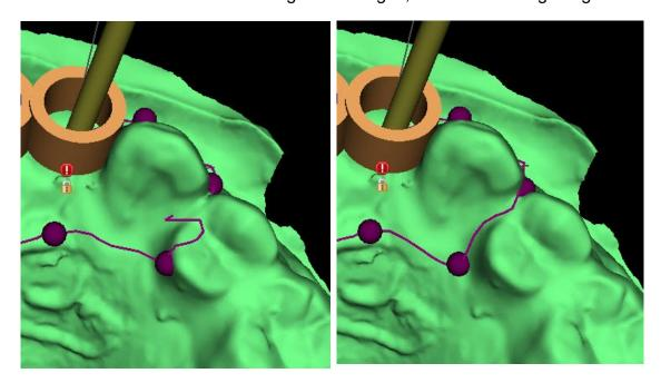
After you finish editing, you can run generation of the surgical guide with button (8). The now unnecessary cropped curve is hidden automatically at this point. This is indicated by the "Show curve" checkbox (7), which can be used to redisplay the curve.
