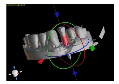
Later on, the scan body position can also be refined manually using the common manipulation widget in the 3D view.
