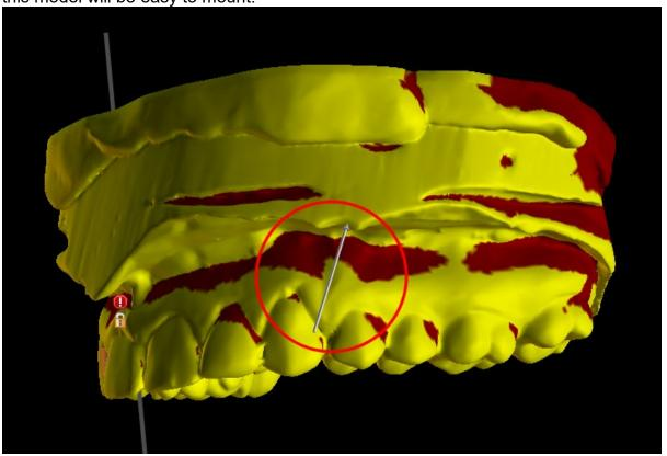
The differences between individual outputs can be compared in the following pair of images. On the left is a guide on the model with undercuts removed; on the right, all details are preserved.
