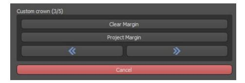
The Project Margin button projects the curve defined by the user on the deformed tooth.
