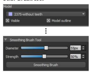
The application provides a basic tool for manually smoothing the resulting surgical guide: the "Brush Tool". This tool smooths the surface, i.e. it lowers bulging parts and evens out depressions. Before using it, ensure that model you really want to edit is selected in (1). If the model is not visible at that given point in time, the program notifies you when you turn on editing mode.
