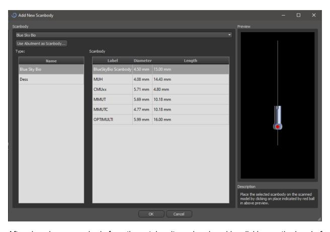
After choosing a scan body from the catalog, it can be placed by clicking on the head of the scanned abutment in the model – for the best fit position, it is good to click on the place illustrated by the red marker as shown in the catalog scan body preview.
