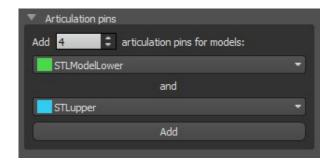
The user needs to select the upper and lower jaw models and click the "Add" button. The number of pins can be changed as well.
