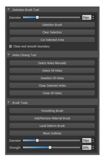
All the necessary tools are available in the Model Edit panel. Using the "Selection Brush" the user can select a part of the surface and remove it by pressing the "Cut Selected Area" button. This way the user can clean the surface from scuttered parts or "extract" a tooth, for example.
