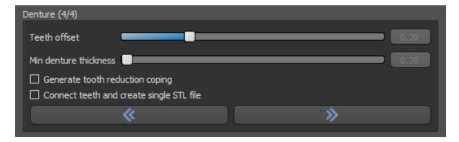
Sliders are used for selecting Teeth offset and Min denture thickness.
