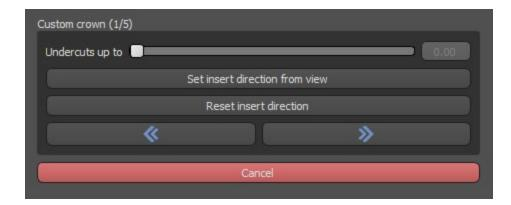
The slider can be used for setting the values for the undercut.
