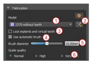
Some input models may be damaged – they are composed of several parts, and their internal structure may not be correct. Fabrication of the surgical guide may fail in these cases. If the input model is damaged, it is possible to try to correct the input geometry using the correction tool (2) and run model fabrication again. When manipulating the model, it is a good idea for the option of working with implants to be
