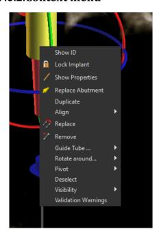
It is also possible to perform several operations on the implant via the context menu, which we can invoke by clicking the right mouse button on the implant.
