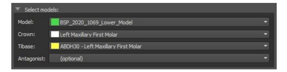
The tibase can be chosen by clicking on the tooth or by clicking on the tibase dropdown. If a tibase is not selected, the user cannot go further.
