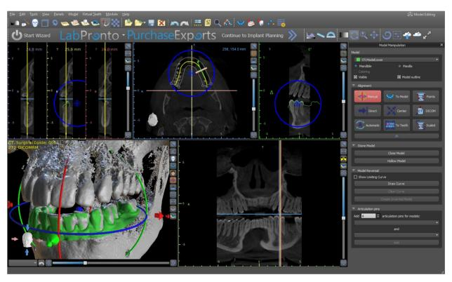
When aligning manually, it is possible to define a fixed point (a so-called pivot) around which the model rotates. In 2D views, the pivot is represented by a cross. By dragging the cross, it is possible to move the model in the plane of view. The model can be rotated using the blue circle. Hold SHIFT and click the mouse button to position the pivot at a different position in 2D views. In the 3D window, the pivot can be repositioned using the small dragger arrows.
