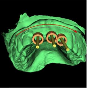
After sketching the basic shape of the surgical guide, switch to border curve editing mode by pressing (6). The shape of the curve can be edited using individual control points on it. Before actually generating a surgical guide, it is a good idea to check its shape in this mode.
