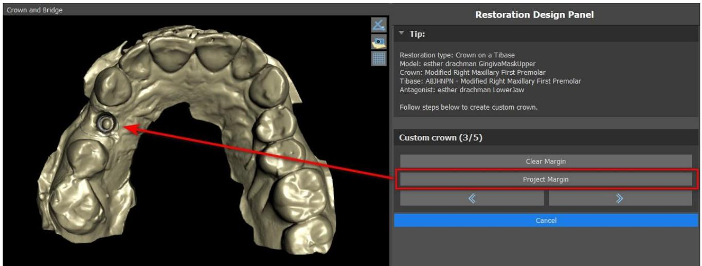
The Project Margin button projects the curve defined by the user on the deformed tooth.
