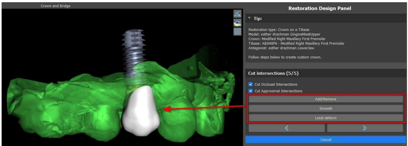
“Add/Remove” is used for the addition/removal of the crown material.
