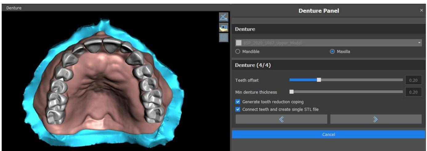
Sliders are used for selecting Teeth offset and Min denture thickness.
