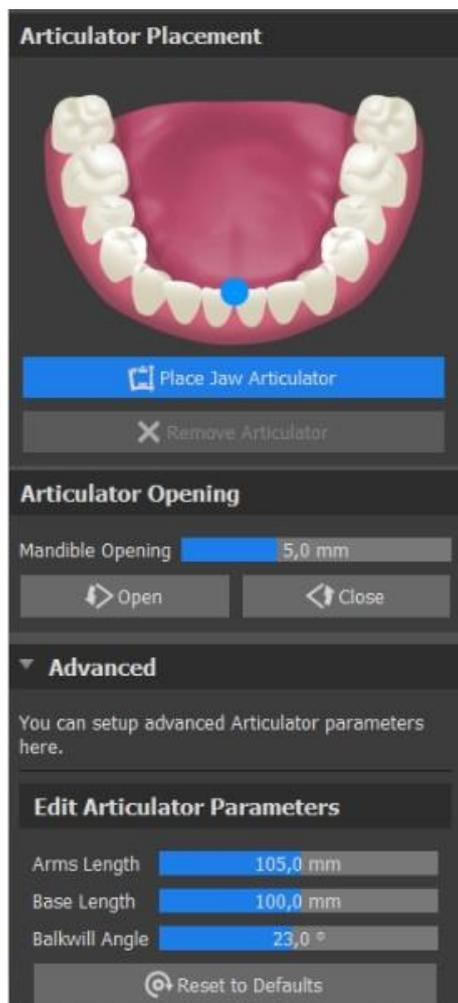
To add jaw articulator, click on the **Place Jaw Articulator** button. The **Remove Articulator** button removes the articulator from the software. The mandible opening slider sets the distance/offset between the jaws. The articulator parameters can be adjusted in the Advanced section. **Reset to Defaults** resets the parameters to defaults positions.
