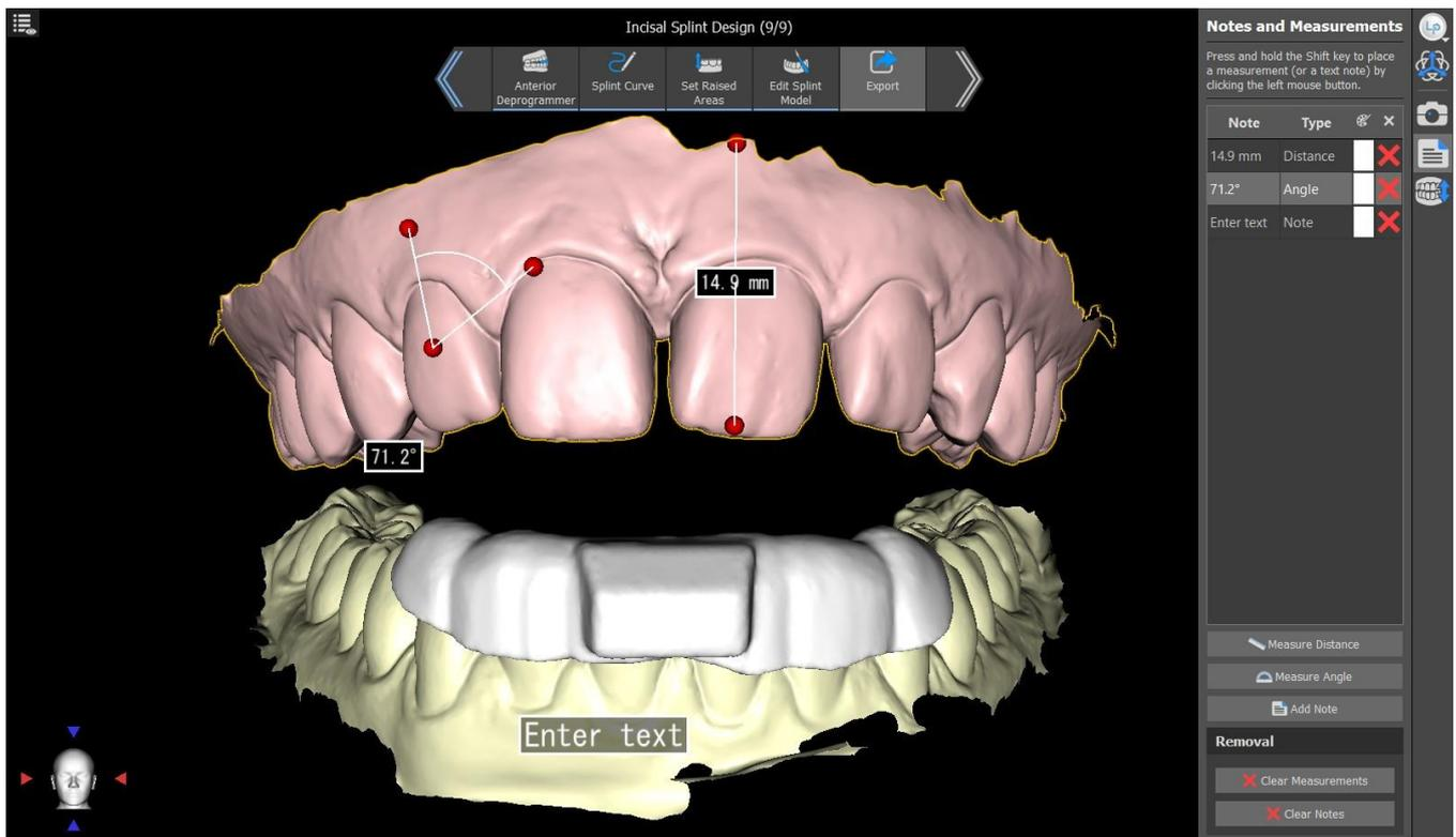
Select the **Measure Distance** button to make any 3D measurements. Click the left mouse button with the pointer on the model to mark the start point of the distance to be measured and click again on the model to mark the end point of the measured distance. To correct the measurement you can grab one of the end points and move them.
