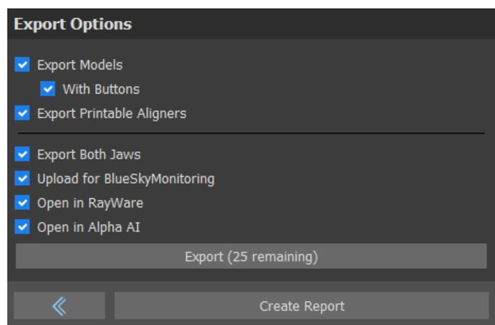
The generated models can be exported from the software in the form of STL models by pressing the “Export” button. By selecting the “Open in Alpha AI”, models can be exported to external slicing software from Ackuretta company. By selecting the “Open in RayWare”, models can be exported to external 3D printing software.
