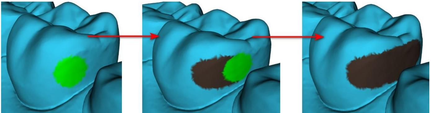
The approximal area can be deleted by selecting “Clear Area”. Pressing the Shift key and holding the left mouse button will define the approximal area and create a brown contour around the selection representing the crown and bridge base. By pressing the Ctrl key and left clicking with the mouse, you can remove the selection.
