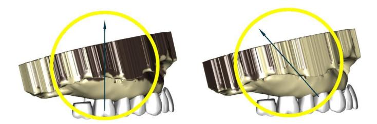
The sliders can be used for setting the values for offset and undercut removal. The insert direction should be adjusted using the rotation ring so that the undercuts are minimised.
