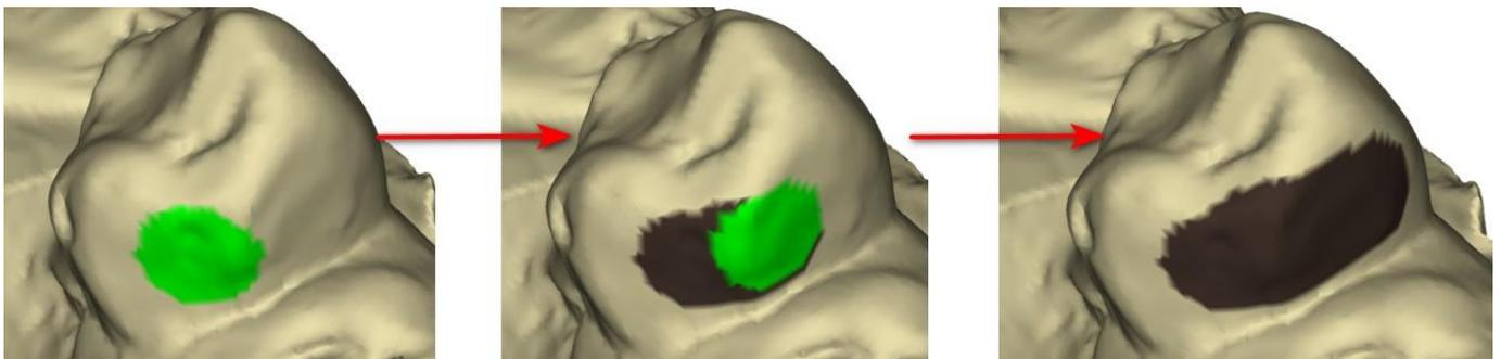
The approximal area can be deleted by selecting “Clear Area”. Pressing the Shift key and holding the left mouse button will define the approximal area and create a brown contour around the selection representing the crown and bridge base.
