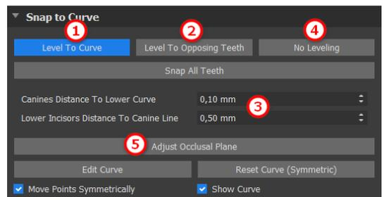
Clicking the "Adjust Occlusal Plane" (5) button activates the occlusal plane for curve adjusting. It is possible to move the plane in the 3D scene based on the angle and distance of the plane.
