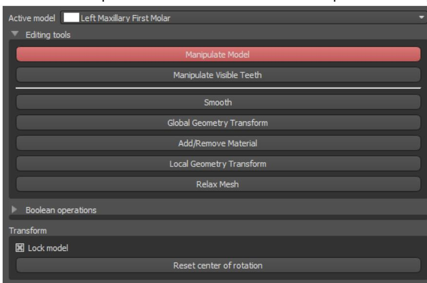
“Manipulate Model” allows the user to change the position of the tooth.
