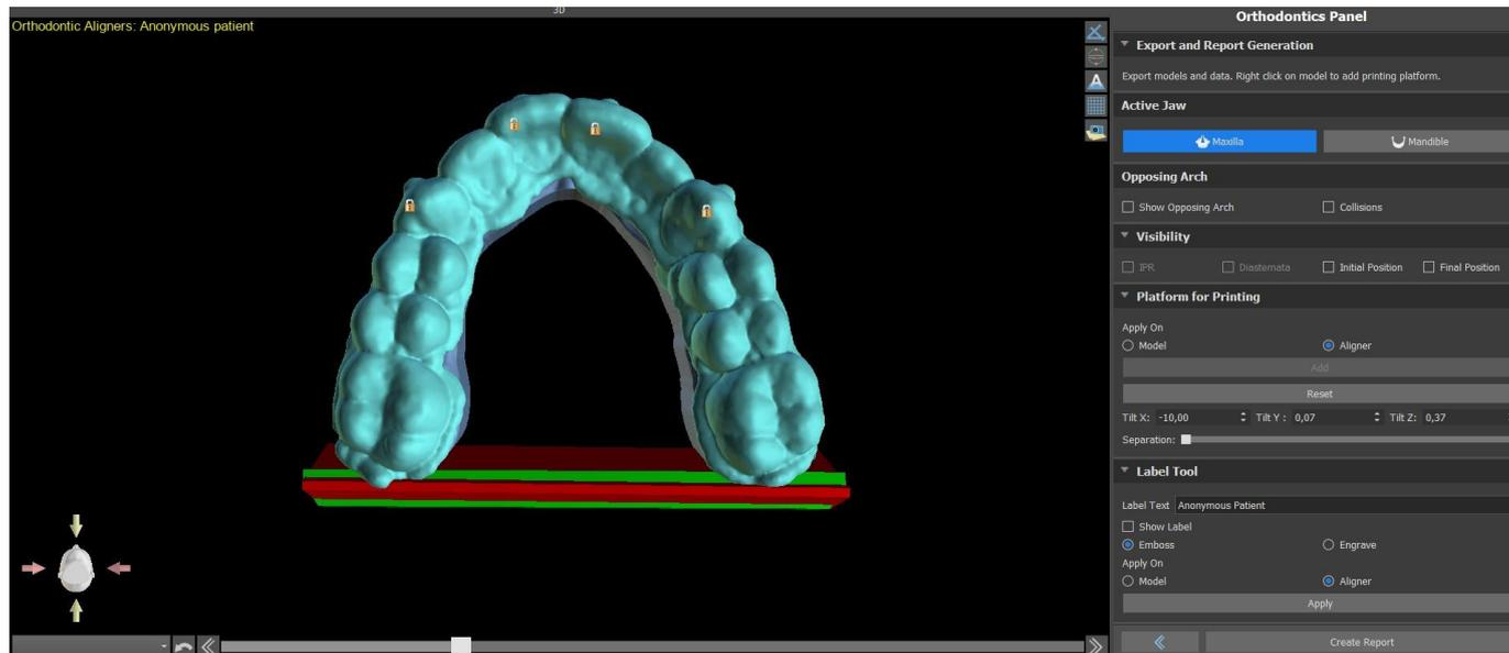
Before the export itself, it is necessary to check all of the intermediate positions of the generated models. After the check, it is possible to export models in different coordinates; regular and separated models can be sent separately. A model's export coordinates can be selected in the Orthodontics Panel.
