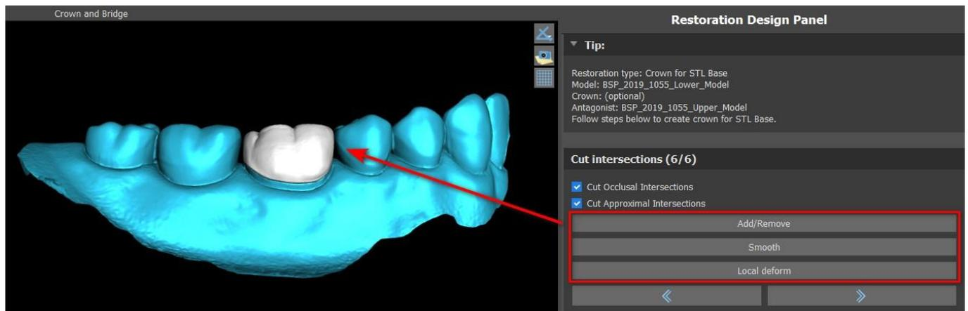
“Add/Remove” is used for the addition/removal of the crown material.
