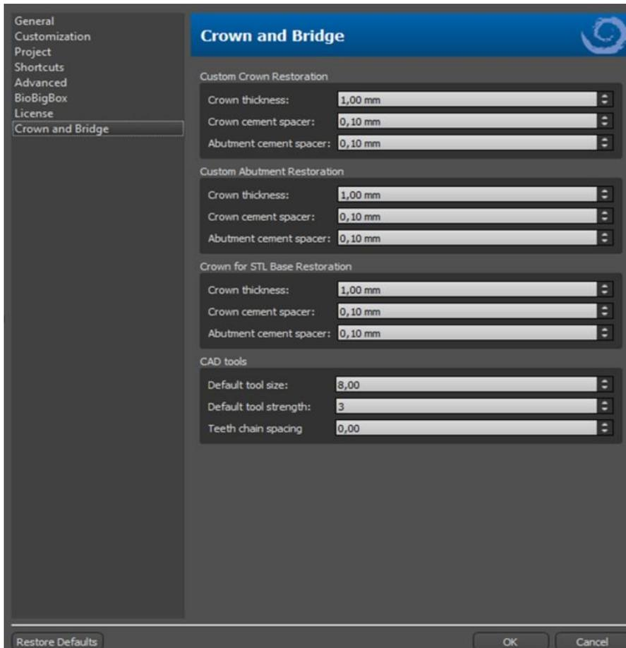
In “Preferences > Crown and Bridge” the user can set the Crown thickness, Crown cement spacer and Abutment cement spacer for different types of restoration available in the Restoration Design panel. CAD tools are available for the Denture module. The “Default tool size” is used for selecting the default tool size, and “Default tool strength” defines the default strength of the tool. “Teeth chain spacing” allows the user to set the spacing between the teeth in the teeth chain.
