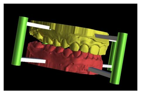
Pins and manipulation widgets will show up. The dimensions of the connecting arms as well as of the pins can be changed by dragging the manipulation widgets which appear when the user hovers over that object. The arrows allow the pins to be moved to the sides and the scale widgets change the thickness of the pins.
