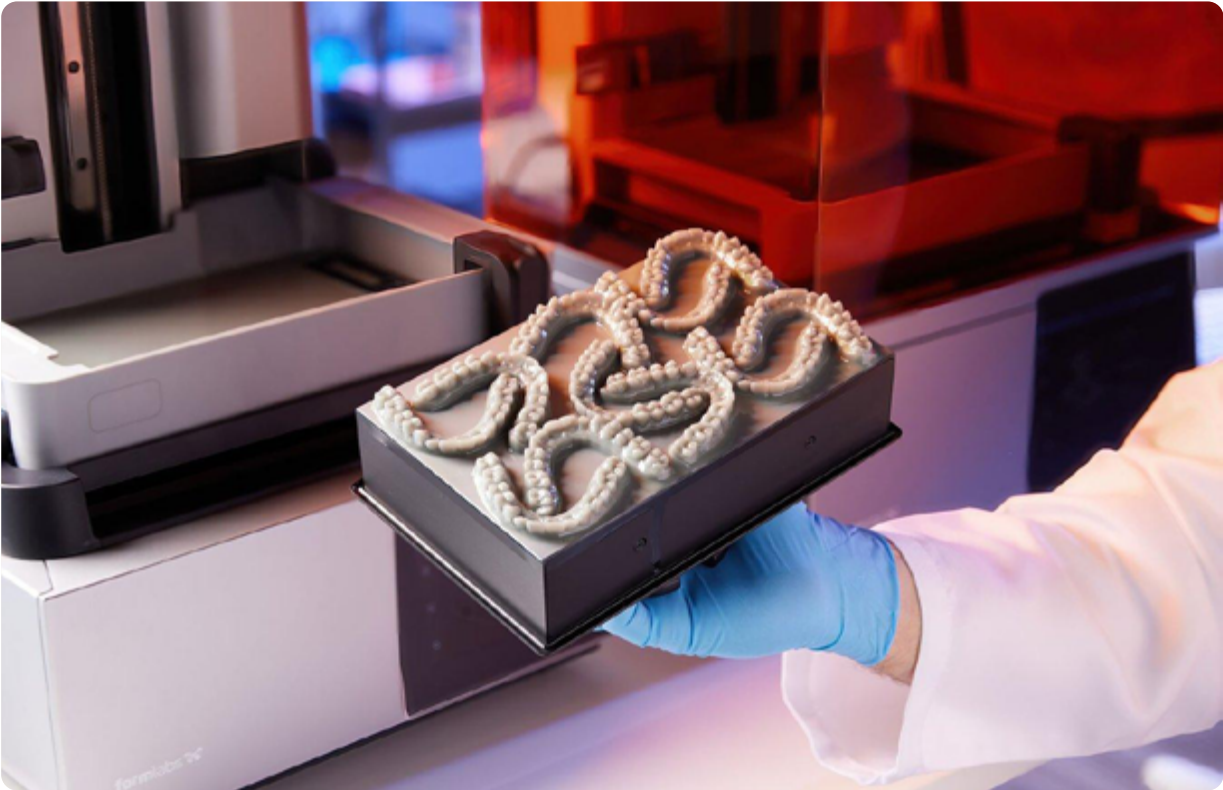
With the LFD Print Engine of Form 4B, surface accuracy is over 95% of data points within 50 µm of the original CAD data consistent across the build platform – while being able to print 11 models in nine minutes.
