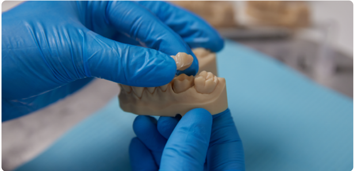
Precision Model Resin is a high-accuracy material for creating restorative models with >99% of printed surface area within 100 \mu m of the digital model.
