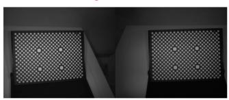
When calibrating, you MUST capture dots right to the edge of the images, so the cameras can be calibrated right to the edge. If you do not, the post scan may never finish because accurate data can never be collected.
