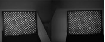
When calibrating, you MUST capture dots right to the edge of the images, so the cameras can be calibrated right to the edge.
