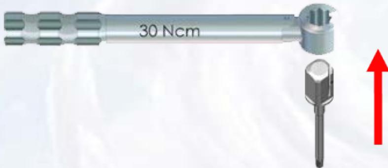
Insert driver into the abutment screw tighten the screw until torque of 30 Ncm is reached and the head of the ratchet releases
