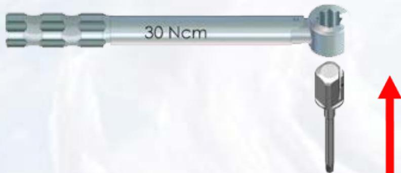
Insert driver into the abutment screw and turn torque ratchet clockwise until torque of 30 Ncm is reached and the head of the ratchet releases
