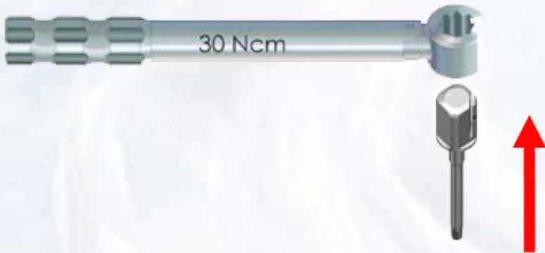
Insert driver into the abutment screw tighten the screw until torque of 30 Ncm is reached and the head of the ratchet releases
